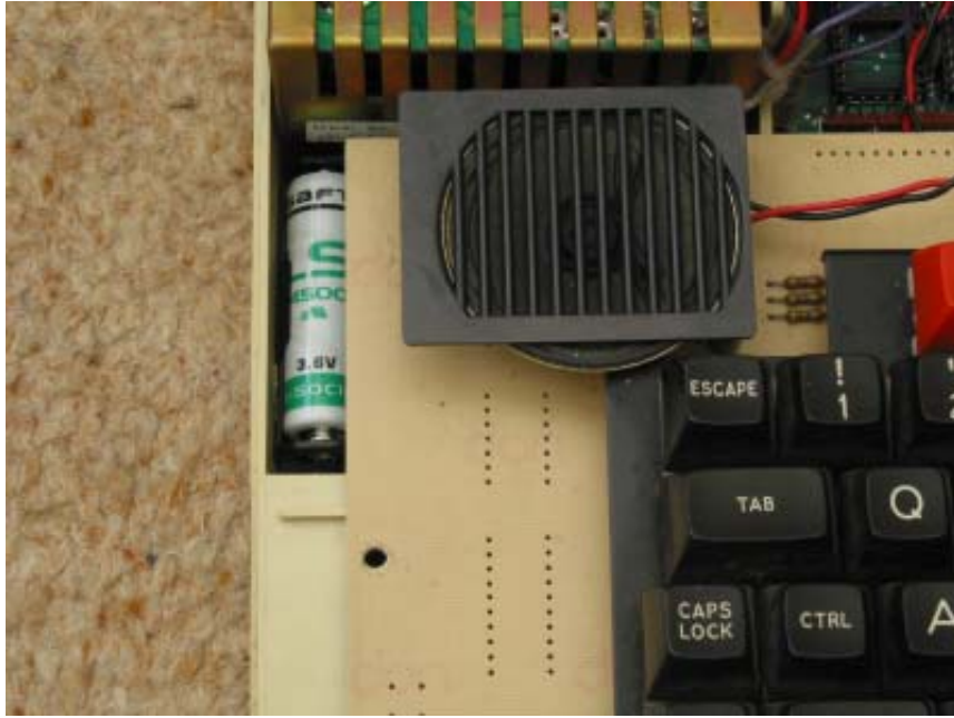
Example installation of a 3.6V lithium thionyl chloride battery in a suitable AA size holder.
